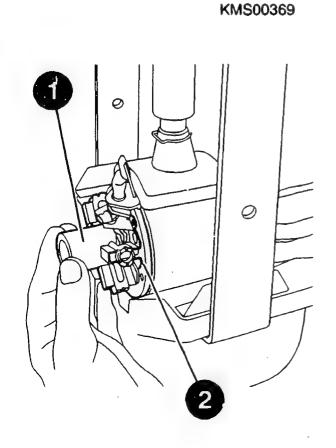
Assembling commutator end shield
